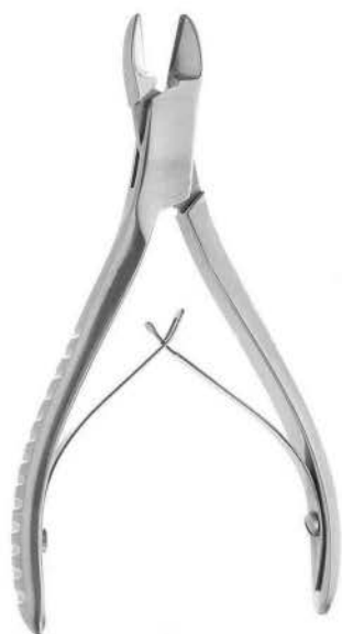
Delicate Wire Cutter S15-885-12 12.5cm Side cutting w/ carbide inserts max capacity. 0.7mm 028"
