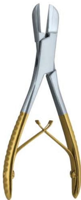
Wire Cutter S15-886-15 15cm for hard wires up to 1mm, for soft wires up to 1.5mm tungsten carbide inserts
