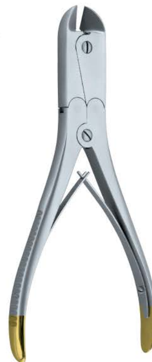
S Line side Wire Cutter S15-893-23 23cm for hard wires up to 2.2mm, for soft wires up to 3mm tungsten carbide inserts
