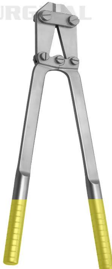
Side Pin Cutter Large S15-922-57 57.5cm Side cutting w/ carbide inserts Max. capacity 6.3mm
