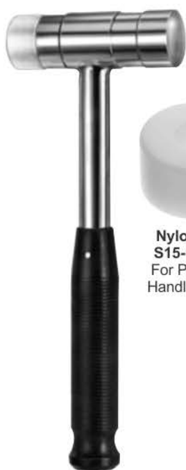
Mallet S15-108-30 26 cm Plane (Nylon) convex (steel) Head 30mm Ø weight 675 grams.
