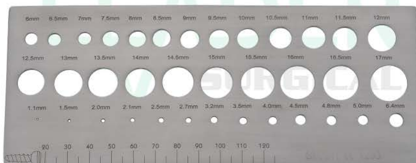
Measuring Gauge S16-326-01 for nail
